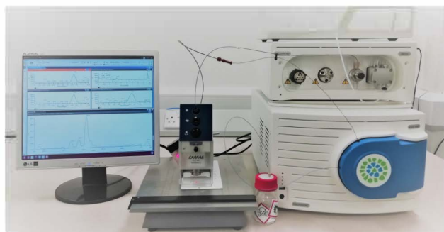
Figure 1. System configuration showing the TLC2 interface connected to the 4500 MiD®
